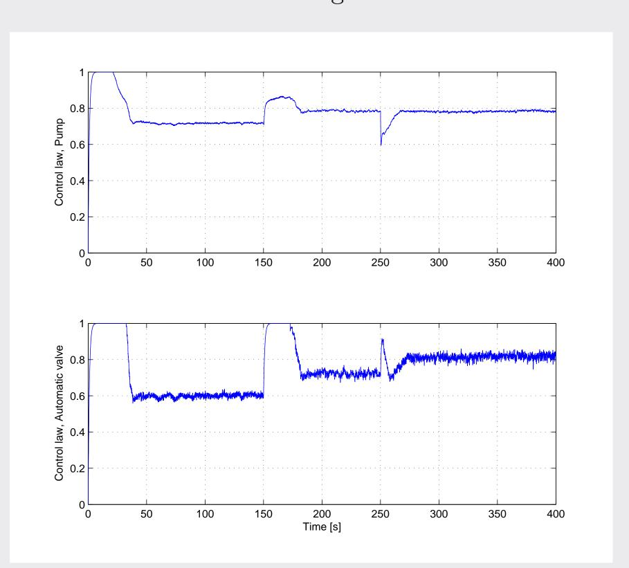
Liquid level control of the TITO system. Control system is capable of tracking reference signals for both tanks.
