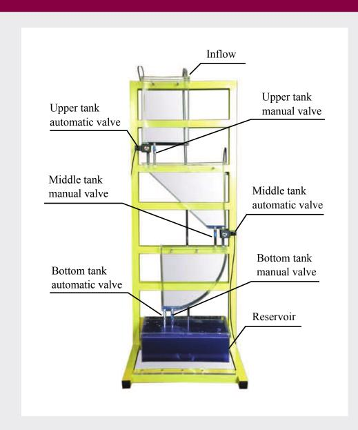
Dynamical behavior of the plant can be described in a continuous time domain by the following differential equations
