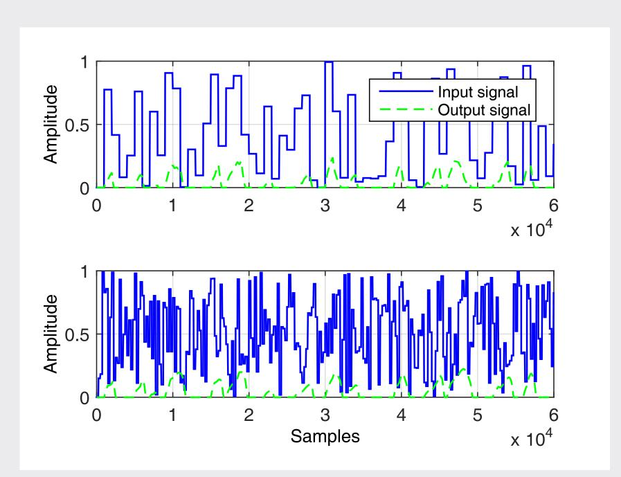
The NN-SANARX structure was trained with 2 neurons on the first and 10 neurons on the second sublayers, the linear and hyperbolic tangent sigmoid activation functions were chosen, respectively. Levenberg–Marquardt training technique was used.
