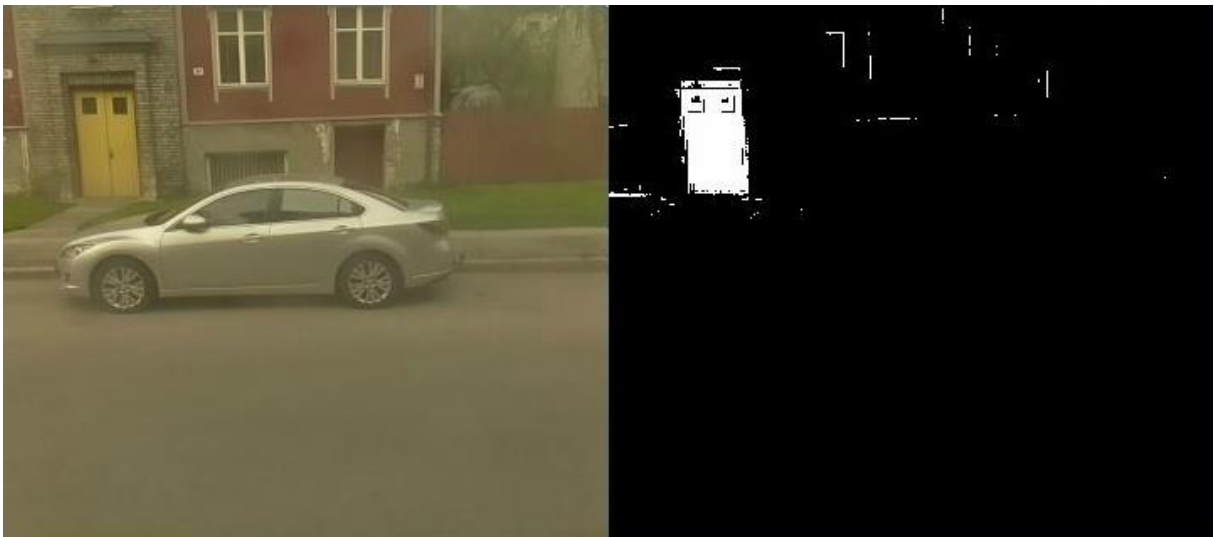
Figure 7. Image after thresholding. The selected hue range in this case was between 0 and 38, which is roughly orange or yellow (colour of door on image). The lower boundary of saturation was also raised to accommodate current lighting conditions.
