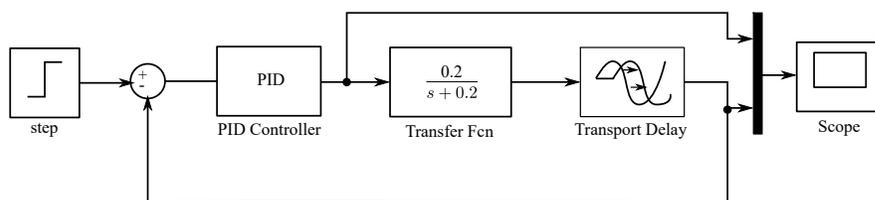
Figure 4: Control of FOPDT plant
