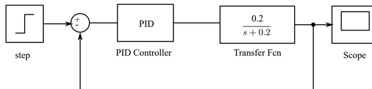
Figure 2: Feedback control of first order plant
