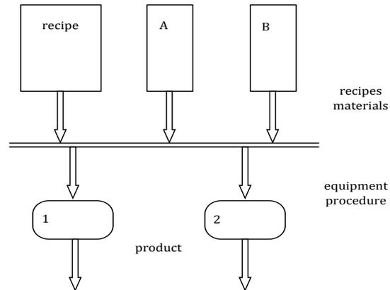
Figure 1.7: Batch process
