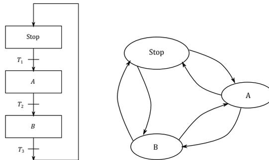
Figure 1.1: State and Data-flow diagrams
