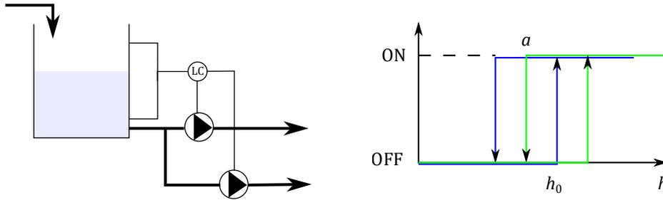
Figure 1.5: Two pumps control
