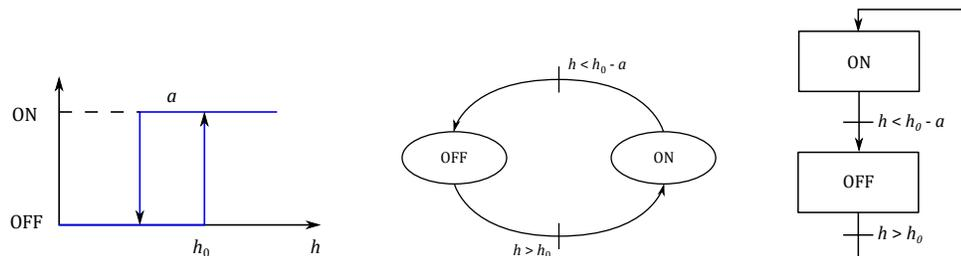
Figure 1.4: Pump On-OFF Control
