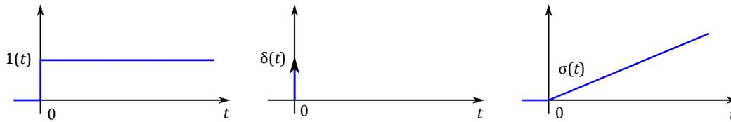
Figure 1.6: Step, pulse, ramp signals
