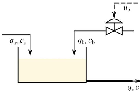
Two liquids  $a$  and  $b$  mixed in order to achieve a concentration  $c$  of substance  $X$ . Outflow concentration is measured (quantity of substance  $X$  in total volume %). Inflow concentrations are  $c_a = 2\%$  and  $c_b = 96\%$ .
