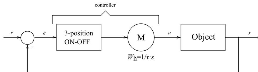
Figure 8: Floating Control diagram
