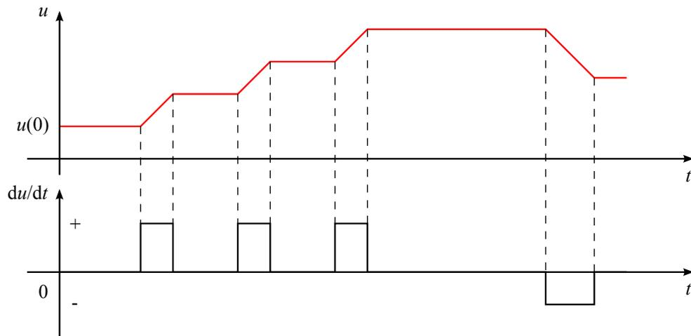
Figure 9: Control process using 3-point controller (floating)
