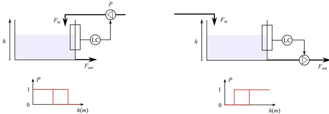
Figure 6: Pumps characteristics
