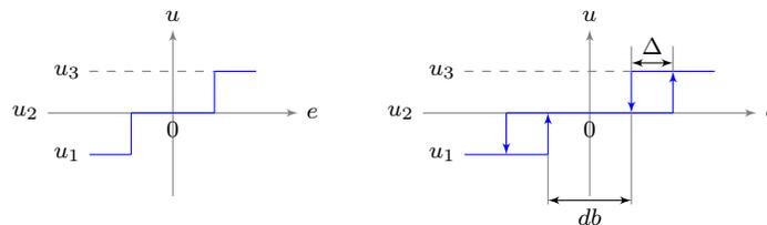
Figure 7: Three point controller without and with hysteresis
