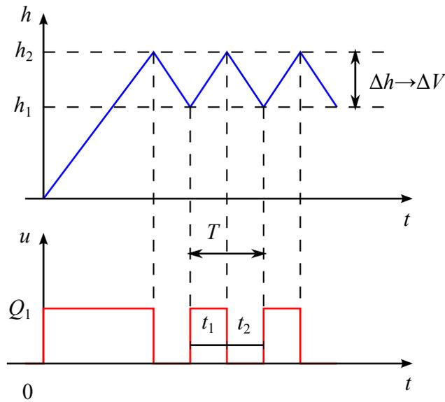
Figure 5: ON-OFF control of integrating object
