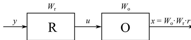
Figure 1: Open-loop Control
