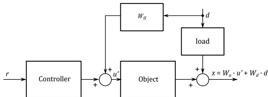
Figure 2: Feedforward Control
