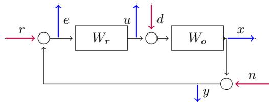
Figure 4: The pure error feedback loop
