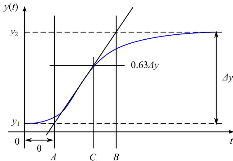
Figure 10: Process reaction curve
